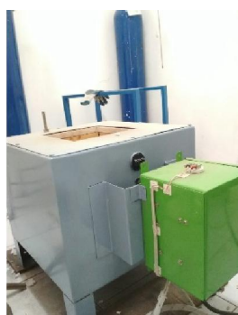
Gambar 2.2 Prototipe TOLACORE apparatus corrosion test
